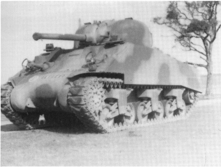
The M4A2 after repainting at Monegeetta. The Australian number can be seen on the transmission housing and the sandshields are already showing signs of damage.
